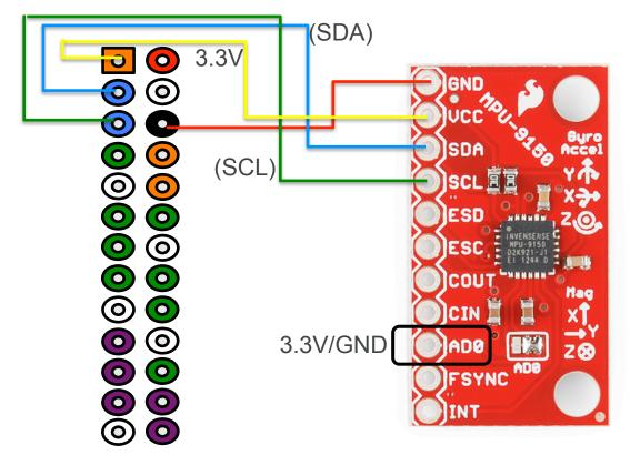
P2 Connector: Pin 1 = 3.3V Pin 7.8 = GND
