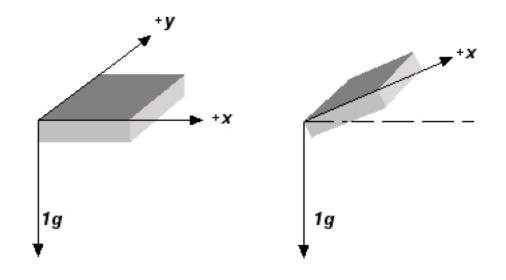
Tilt Angle using One Axis Sin-1 (a)
